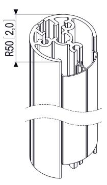
The PUC 2115 is equipped with a double CIS® cable duct system with which you can quickly and simply ensure that all cables are concealed. The pole is made of aluminium and, therefore, it can be easily cut at the required length. Therefore, combine a pole with one of the Connect-it ceiling plates (PUC 1010, PUC 1030 or PUC 1040) or the truss adapter (PUC 1050) and a Connect-it interface (PFI 3010, PFI 3020 or PFI 3030) for a complete ceiling solution.
