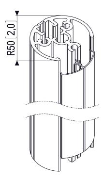
The PUC 2108 is equipped with a double CIS® cable duct system with which you can quickly and simply ensure that all cables are concealed. The pole is made of aluminium and, therefore, it can be easily cut at the required length. Therefore, combine a pole with one of the Connect-it ceiling plates (PUC 1010, PUC 1030 or PUC 1040) or the truss adapter (PUC 1050) and a Connect-it interface (PFI 3010, PFI 3020 or PFI 3030) for a complete ceiling solution.
